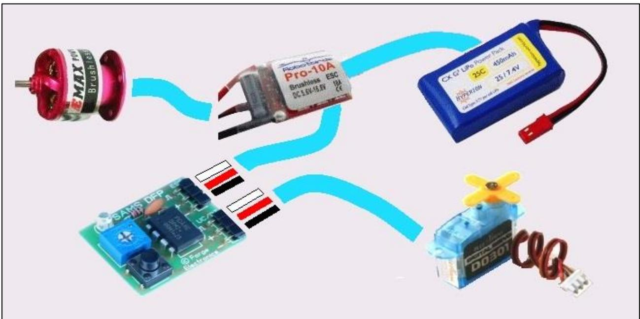
The signal lead from the ESC, usually coloured white/red/black, connects to the top three pin header on the timer as shown in the image above and the U/C servo to the lower three pin header. Note the orientation of white/red/black leads.
